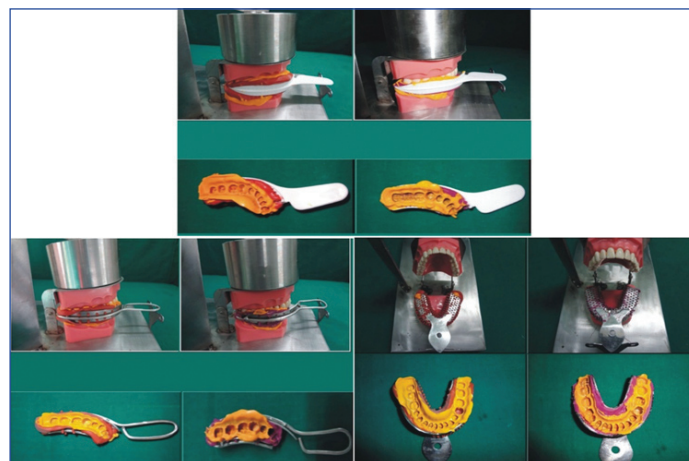
[Table/Fig-3]: Impression making and completed impressions of rigid and monophase impression materials with light body in three different type of trays.
